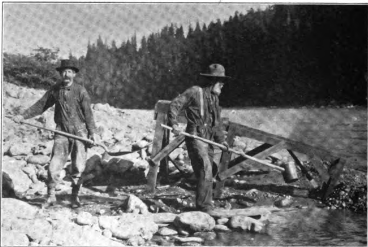
Fig. 40. Long Tom operated successfully by A. M. Collins and G. W. Way on the bank of Rogue river at Agness
