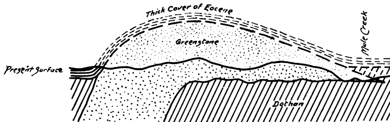
Fig. 15. Suggested section (idealized) through the greenstone intrusion west of Mule creek
