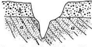
FIGURE 11.—Section of tailrace of Logan mine. *a*, Cretaceous sandstones, shale, and conglomerate; *b*, gravels of third cycle of erosion.
