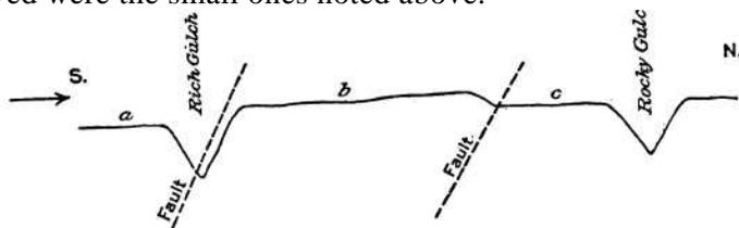
FIGURE 19.—Profile of old-channel bedrock in Harvey mine. Arrow shows course of ancient stream. Bedrock at *a* is 30 feet lower than that at *b*, whereas at *c* bedrock is 15 feet lower than that at *b*.
