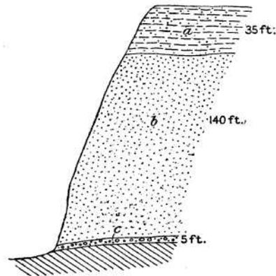
FIGURE 18.—Section of gravel in Old Channel mine, south of Rich Gulch, *a*, Clay and sand; *b*, fine gravel, well rounded; *c*, coarse gravel, containing cobbles as large as 8 inches in diameter but few bowlders.
