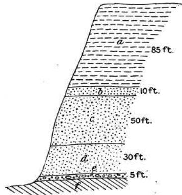
FIGURE 17.—Section of gravel in Old Channel mine, north of Rich Gulch, *a*, Red earth and clay; *b*, gray sand; *c*, gravel and sand; *d*, fine gravel; *e*, bowlder bed and coarse gravel; *f*, slate
